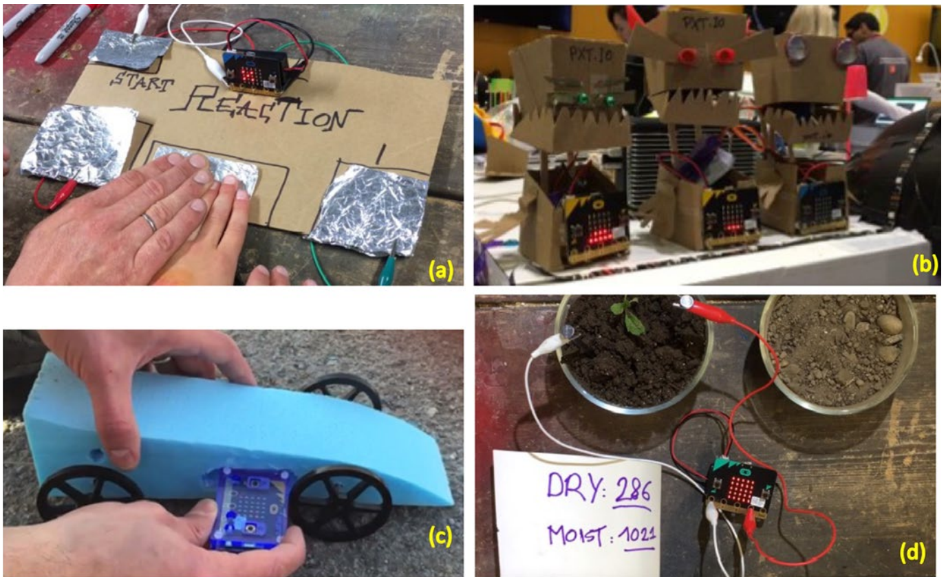
Figure 5: Example projects: a) the reaction game; b) light-reactive cardboard robots; c) a Bloodhound model rocket car instrumented with a micro:bit; d) measuring soil moisture via micro:bit pins 2 .
